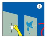
Make sure surface is clean, free from grease, oil, dust/dirt or any other surface contaminants.
