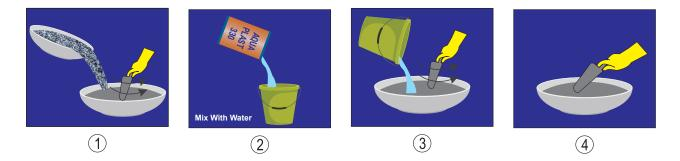
**DOSAGE:** Field trials should be conducted to determine the optimum addition rates of Aqua Plast 330. A dosage range 280cc to 560cc per 100 kg cement is recommended as an initial starting point. For hot whether concreting where Aqua Plast 330 is to be used to extend workability, a dosage of 400cc to 500cc per 100kg cement is recommended.
